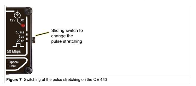
With pulse stretching connected, the individual pulses of a burst event are combined in one 50 ms signal and output on the BNC socket. This pulse stretching prevents devices with high dynamics (counter) from detecting individual pulses of the burst event (a pulse package of a duration of 15 ms is counted as one burst).
