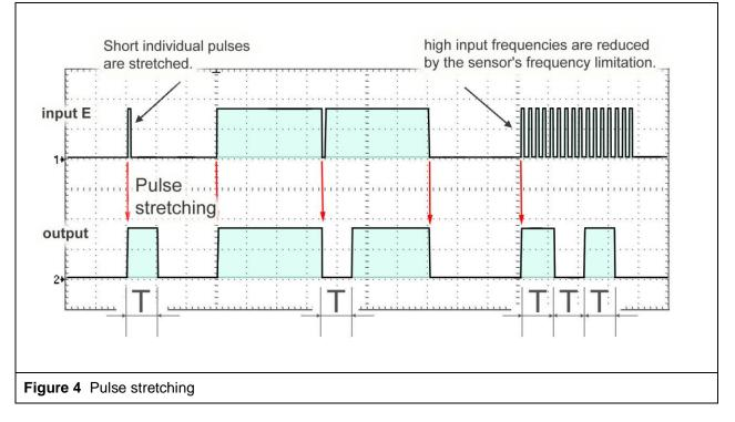
Very narrow input pulses are stretched to a transmissible width (approx. 20 ns) for transmission via synthetic optical fibre. It is thus possible to detect burst or ESD pulses that directly couple in the line connected to the sensor input.
