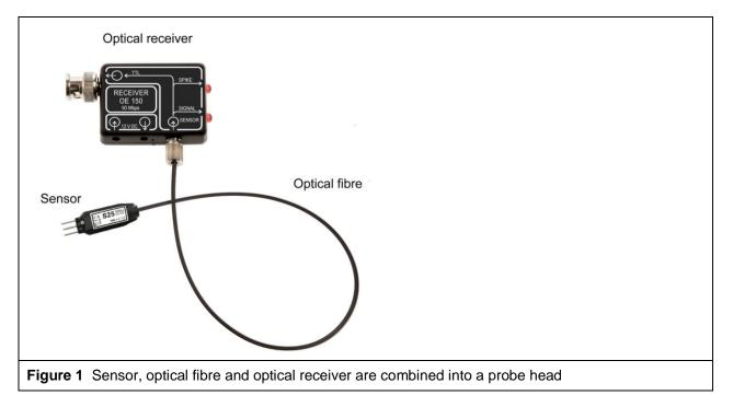
The sensors also contain a pulse stretcher. This stretches short input pulses that cannot be transmitted directly due to the limited band width of the optical fibre to a transmissible pulse width.
